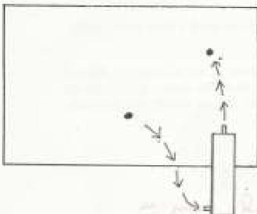
AN EXAMPLE OF CORRECT INSTALLATION. NO DIPS OR LOOPS IN HOSE. THERE IS A HEAD OF WATER IN THE BLOCK ABOVE THE TOP CONNECTION TO ALLOW HOT WATER TO RISE WITHIN ENGINE
